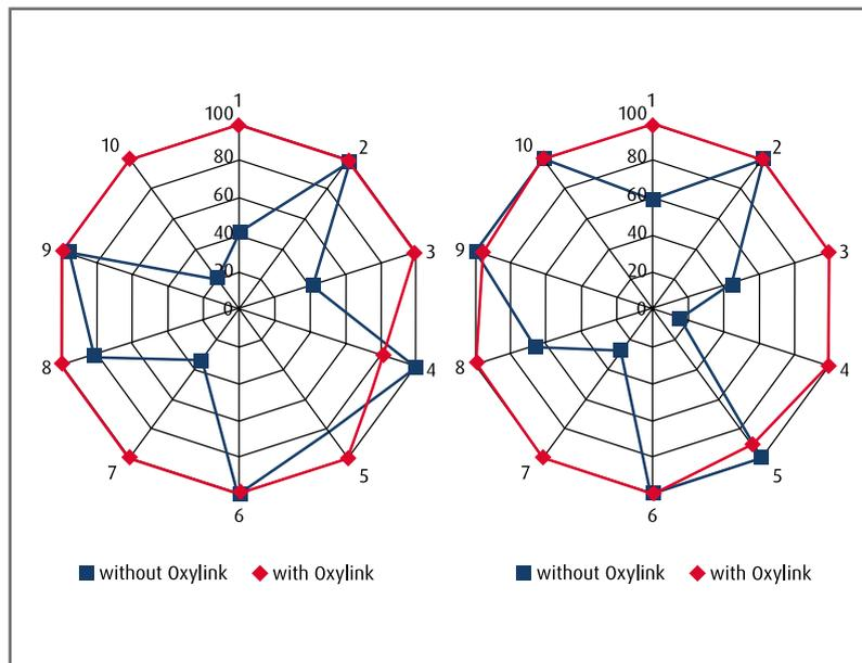
Figure 5: Left: Performance diagram of HBST formulation with and without nanoparticle additive. Right: Performance diagram of WG formulation with and without nanoparticle additive
